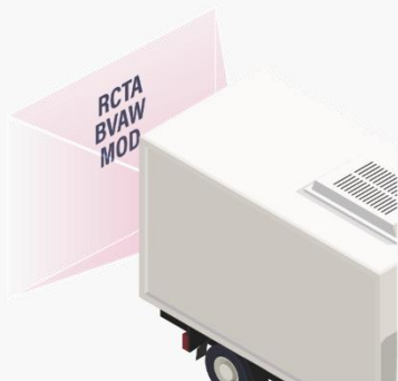
RCTA Rear Cross Traffic Alert BVAW Backward Vehicle Approaching Warning MOD Moving Object Detection
